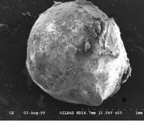
Fig4.3. (a) Scannig electron micrograph of TM loaded NMS microbead at 5x.
